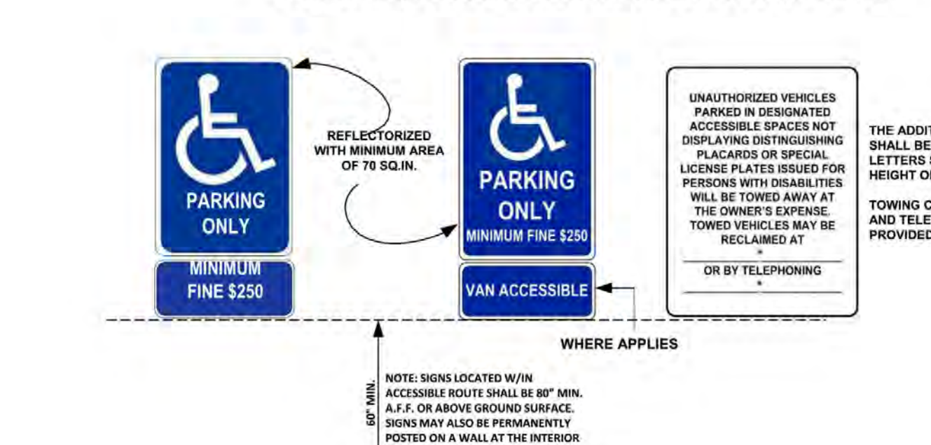
FIGURE 11B-502.6 ACCESSIBLE PARKING SIGN INSTALLED AT EACH SPACE
