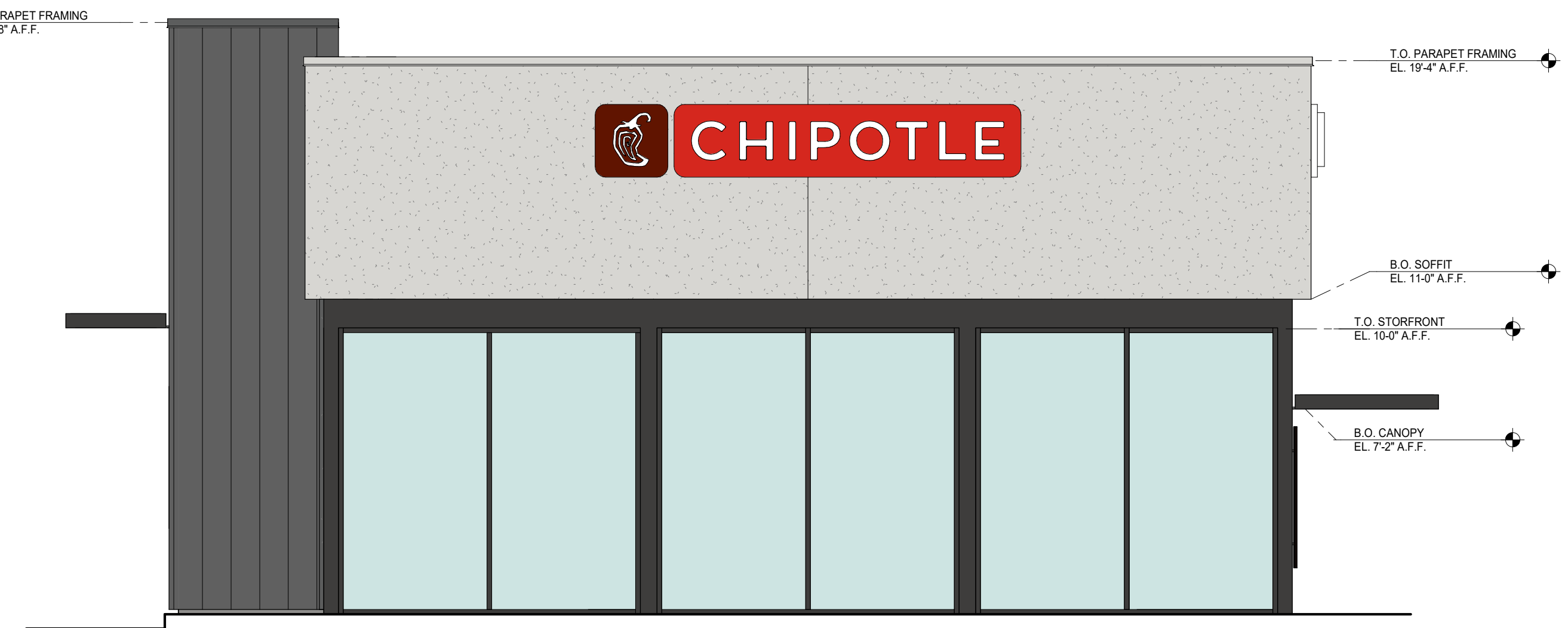
② EXTERIOR ELEVATION - EAST 1/4" = 1'-0"
