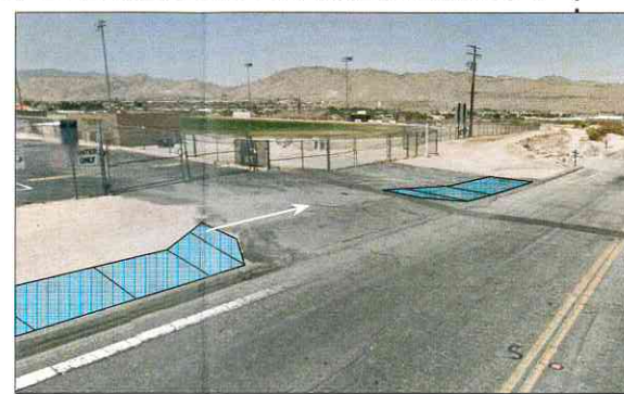
Proposed sidewalk will have a gap with transitions at the existing north AC driveway on the northernmost YVHS parking lot, located adjacent to the fields.
