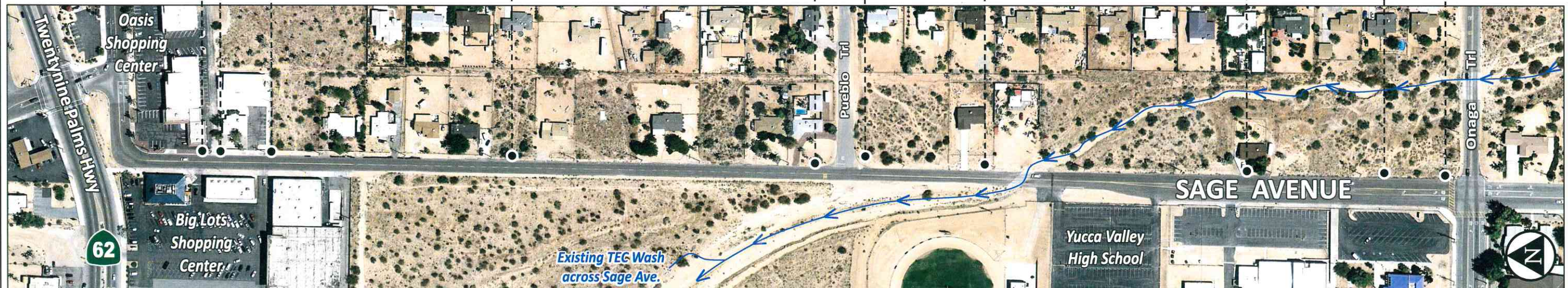
NEC of Sage Avenue at Jamie Ann Lane. Full width of sidewalk to be constructed with ramps at Jamie Ann. Some relocation of signage may be required from the alleyway to Yucca Trail with utility protection.
