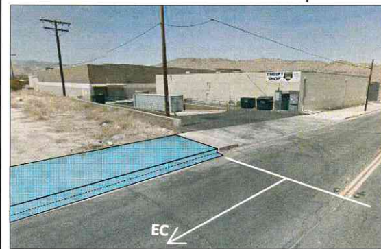
Proposed sidewalk/C&G shall connect to and match the existing sidewalk along the east side of the existing retail center, at the southeast corner, to a full 60" width.
