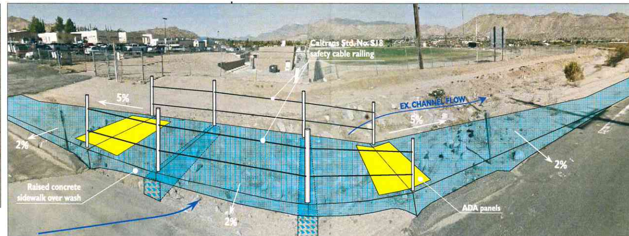
Our proposed alternative would involve the design of a raised concrete sidewalk over the existing TEC crossings on each side of Sage Avenue. The slightly elevated pathway would allow the natural drain wash to continue to flow over the street. Caltrans cable railing would also be installed for fall protection along the sidewalk length.
