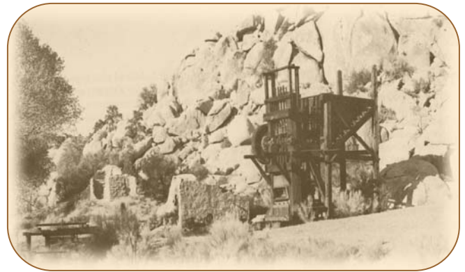
Example of Stamp Mill at Desert Queen Mine in Joshua Tree National Monument Source: Yucca Valley Reflections of the Past
